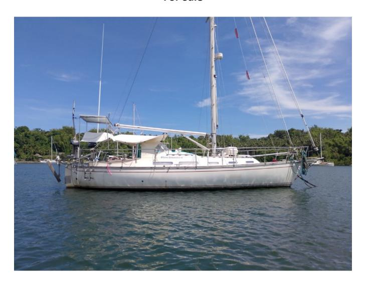
This world cruiser has full keel and is built of solid fiberglass. The boat has main sail with 2 reefs, double furling headsails and two whisker poles. The boat can be sailed downwind with the headsails opened on both sides, which gives easy control from cockpit.
